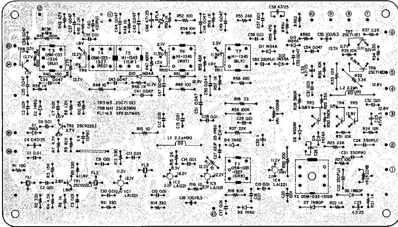
Fig. 6 FM-AM IF AMP. P.C. BOARD 94-5009 (Rev. Side)
